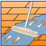
**Grout residues:** remove cement based grouting residues and building dirt's by washing the floor with Lithofin KF Cement Residue Remover. Dilute the product approx. 1:5 and apply generously to the surface. Scrub well with a broom or scrubbing machine and allow another 10 minutes working time. Add water before scrubbing again. Then take up dirt deposits and product residues with a wet vacuum before rinsing the surface with plenty of clear water. On small areas use a brush or white nylon pad.
